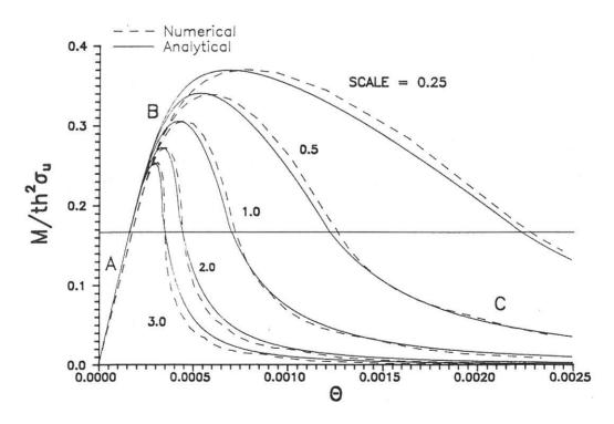
Figure 2: Moment rotation curves obtained through the numerical method together with the analytical ones.
